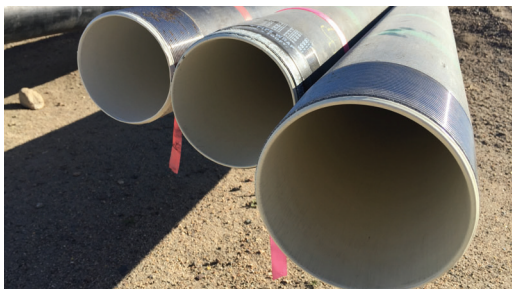
150,000 liner feet of pipe applied with Denso Archco™ 453HTP and 466P.
