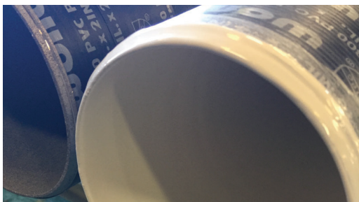
Finished Archco™ 453HTP & 466 pipe lining applied.
