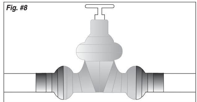
7.5 The final tape wrap starts on the top of the center of the flange and overlaps onto the previous tape. Working away from the flange onto the connected pipework in a vertical motion, the tape is applied using a 55% overlap to give a double thickness. This application is repeated on the other side of the valve to complete the wrapping. Smooth down the tape and its edges to remove air and form a seal (See fig #7).
