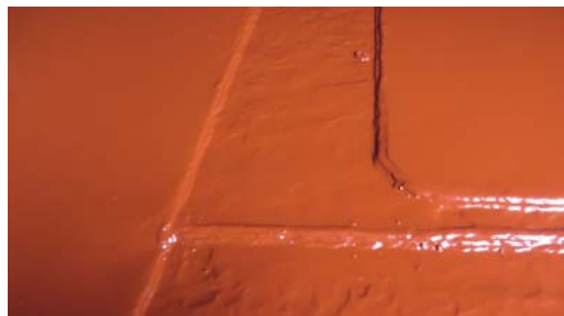
400 wets out and penetrates the anchor profile and heavy pits.
