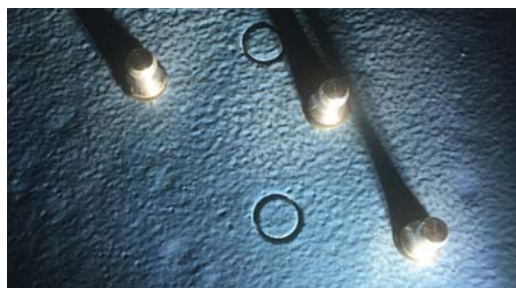
Adhesion test, 2500 psi to 2800 psi
