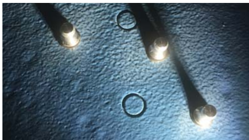
Adhesion test, 2500 psi to 2800 psi
