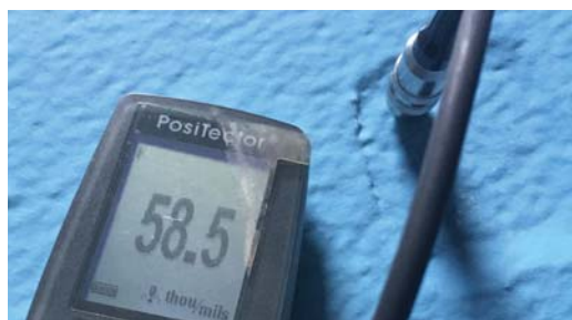
System 400 primer @ 4 to 5 mils dft, 30 to 35 mils dft of 476F single leg.
