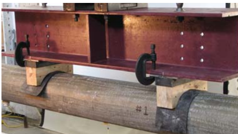
Bending test setup & actuator for the SeaShield Series 400.
