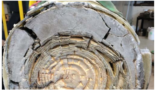
All specimens withstood 3 to 4 times the failure load of the baseline control specimen.
