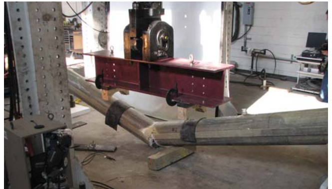
SeaShield Series 400 System at least doubles the maximum load than an undamaged, unprotected timber pile.
