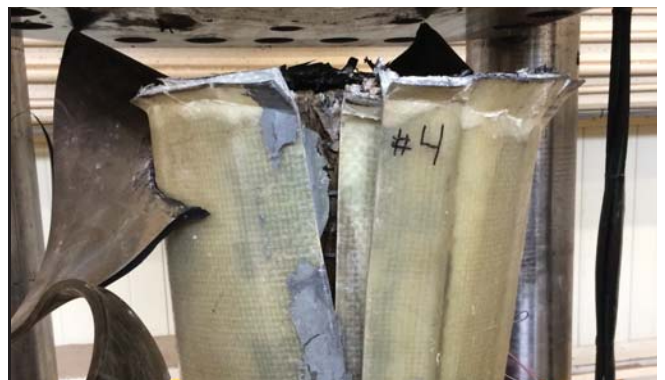
Timber piles installed with the SeaShield Series 400 System were able to withstand a maximum compressive pressure up to 466.6 kips.
