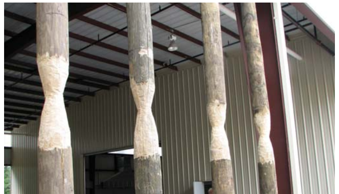
Simulated timber pile hourglass deterioration prior to having the SeaShield Series 400 System installed.
