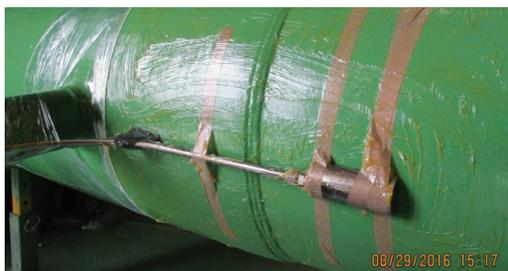
RTD Sensor attached to Protal 7200 coated pipe and a thin layer of Denso Paste HT coating the sensor.
