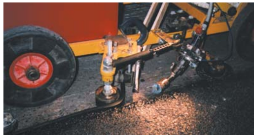
Close up of the Densoband applicator machine.
