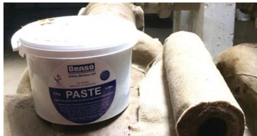
Denso Paste and a roll of Denso LT Tape are used to provide corrosion protection to surface substrate.
